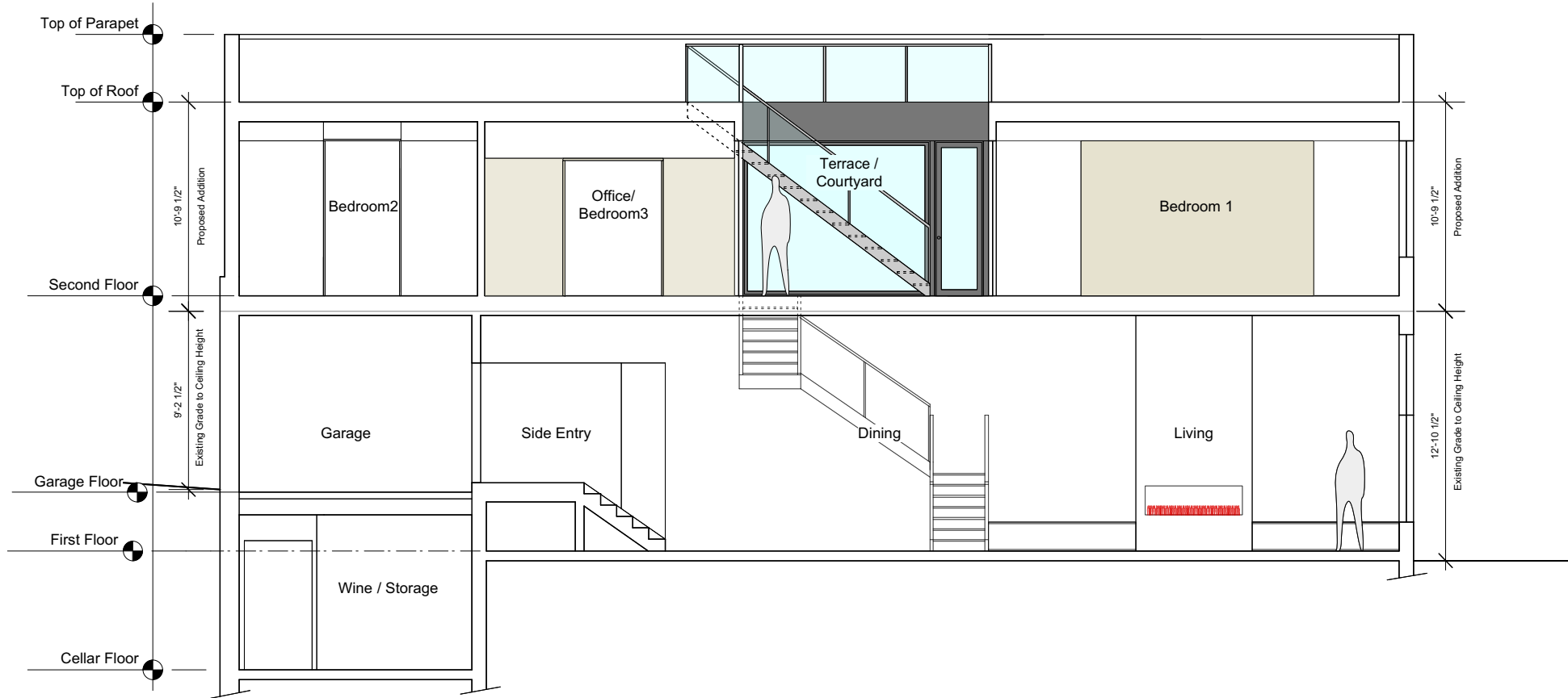
○ Proposed Building Section 2 scale: 1/8" = 1'-0"
